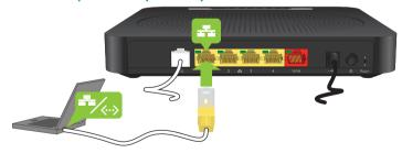
If you want to connect a device using a wired (Ethernet) connection:
